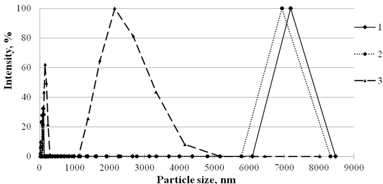
**Fig.4.** The graph of the distribution of the particle size of the dispersed phase of the initial phase and the filtrates of the "methylene blue" model solution (1-model dye solution, nylon membrane filtrate, nylon-gelatin membrane filtrate).
