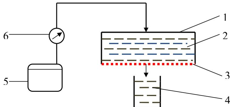
**Fig.2.** The diagram of laboratory unit for membrane separation: 1 - membrane module, 2 - model dye solution, 3 - microfiltration membrane, 4 - receiving capacity of filtrate, 5 - compressor, 6 – manometer.
