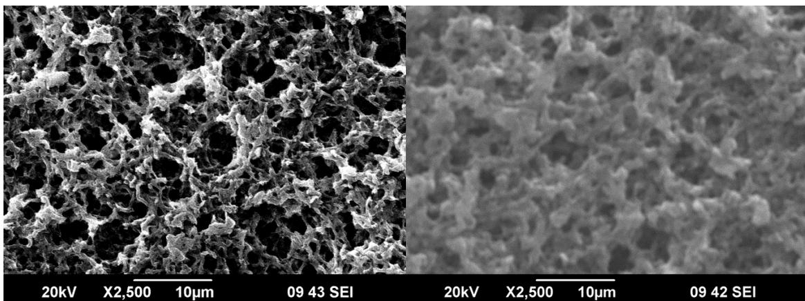
**Fig.3.** Morphology of surface of the original nylon membrane in an increase of 2500 times (left) and modified nylon-PANI membrane in an increase of 2500 times (right).
